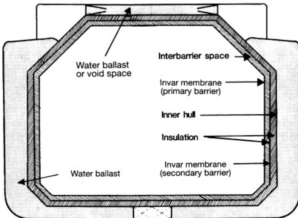
Slika 15. Presjek spremnika GazTransport Cargo Containment No 96
