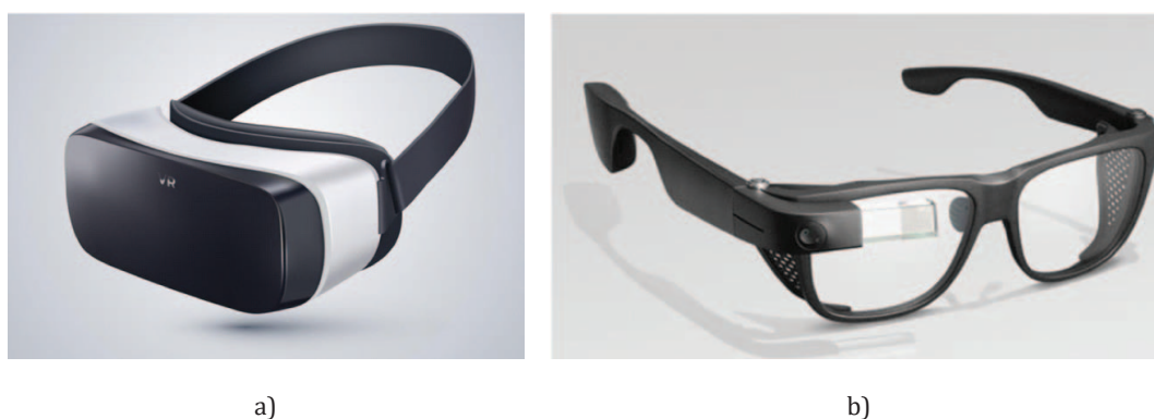
Fig. 3 Example of: a) VR, b) AR headset. Note the complete (VR) and partial (AR) immersion in virtual reality while wearing headsets.
