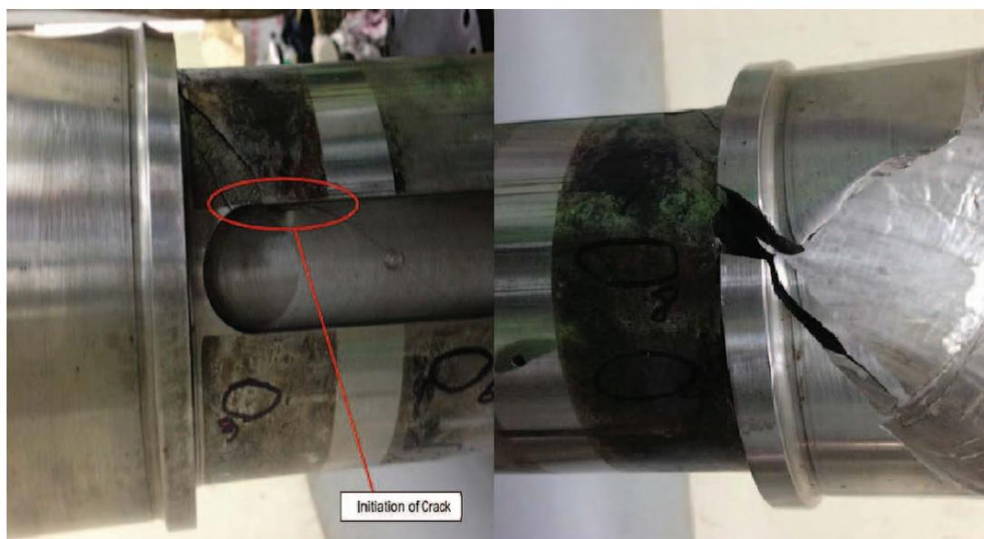
Figure 3 The Characteristic Torsional Failure Crack Shape [8]
