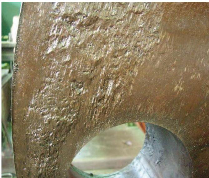
Figure 6 Fatigue Indicative Fretting on Surfaces [13]
