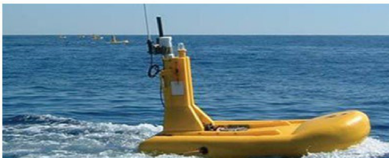
Figure 6 - Seismic tail buoy [17]
