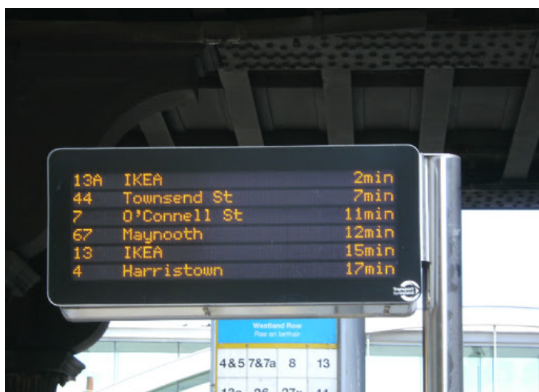
Figure 2 – Display of the RTPI system notification screen in Dublin Source:[11]
