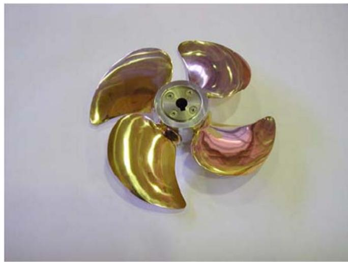
Slika 167: CPP propeler s broda RV Nawigator XXI [4]
