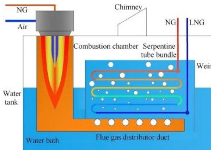
**Slika 14: Submerged Combustion Vaporizer**
