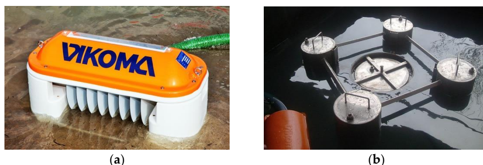
Figure 3. Disc skimmer (a) and weir skimmer (b) [11].
