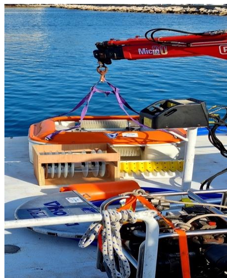
Figure 7. Testing efficiency of brush and disc skimmer [Authors].
