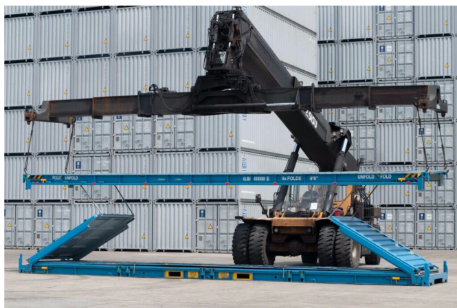
Figure 9 The folding process of the 4FOLD container [1]
