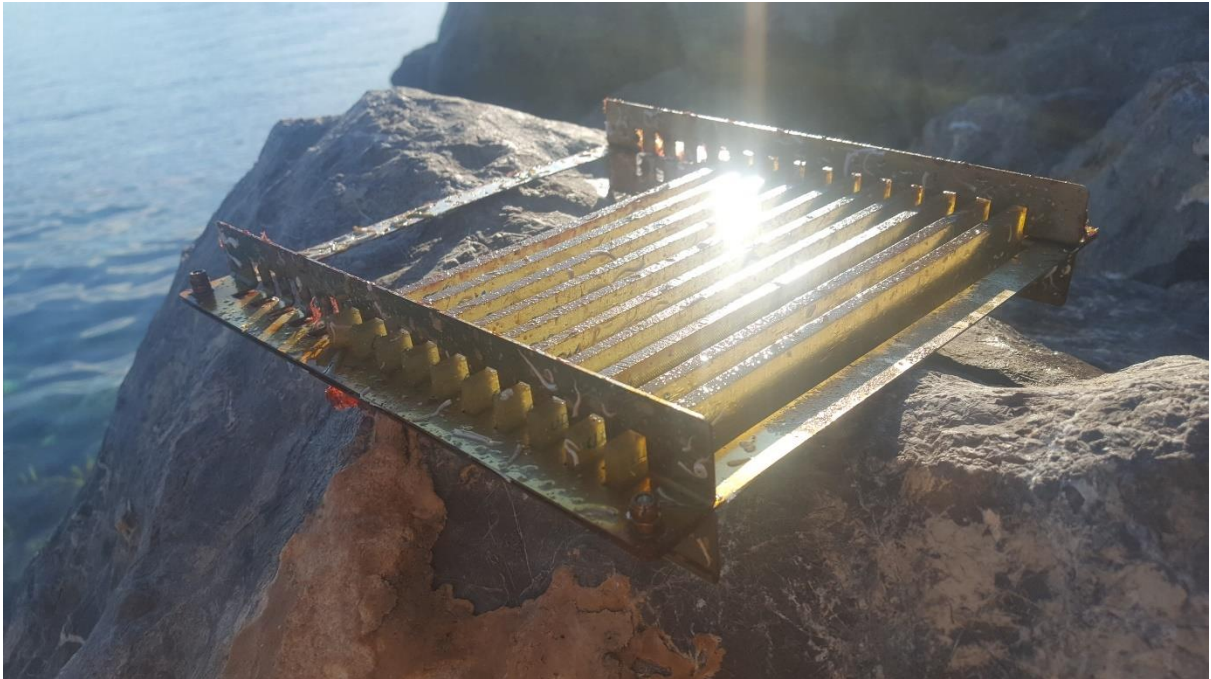
Figure I.6 Coupons in frame after 6 months of submersion
