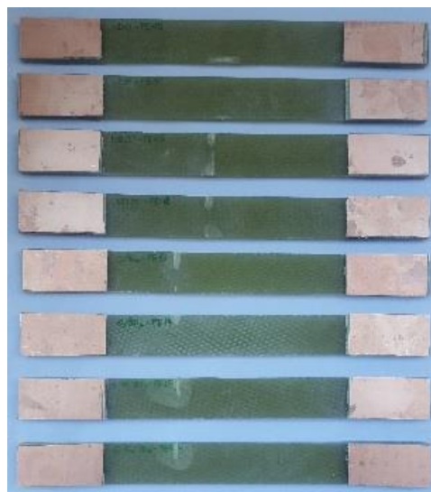
Figure I.4 Coupons with tabs before submersion
