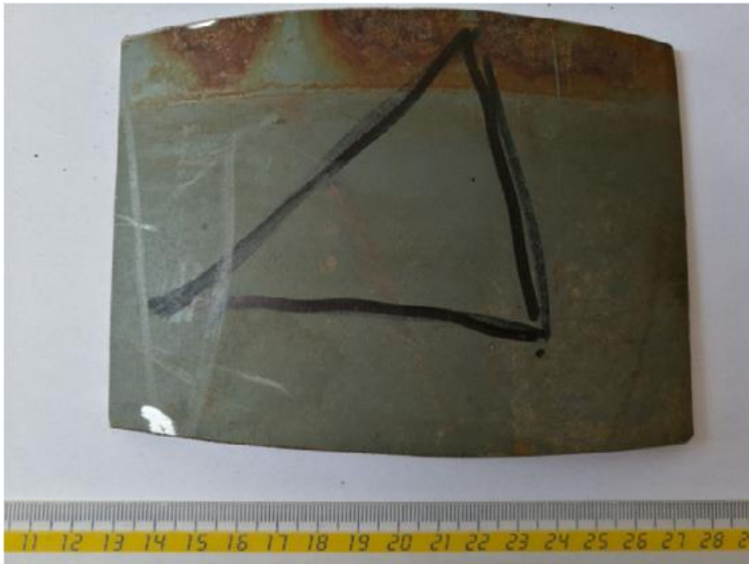
Fig. 4. Cut-out specimen containing crack used to perform microscopic examination.
