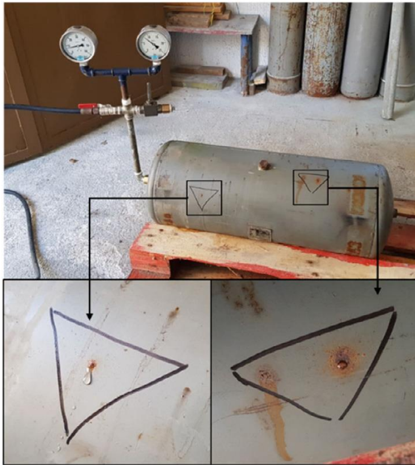
Fig. 2. Hydrostatic test setup with details of fluid leakage.
