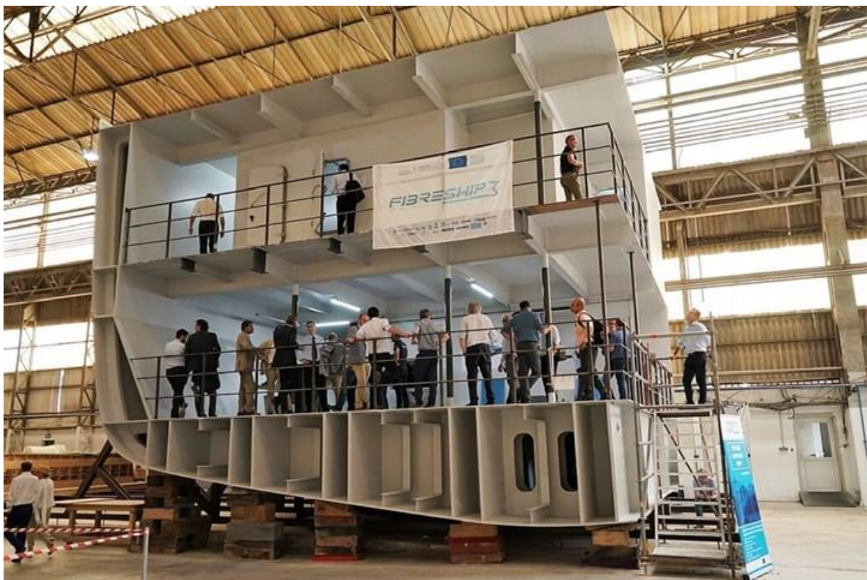
Figure I.1 Composite ship hull section (source: http://www.fibreship.eu/fibreship-2nd-public-workshop/ )
