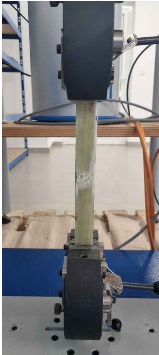
Figure I.7 Coupon on completion of the tensile test
