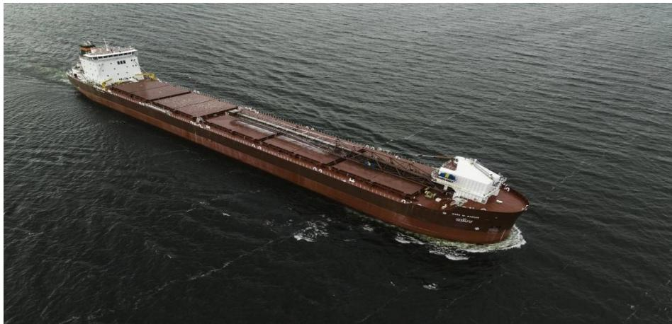
Slika 8: Bulker Laker Mark W. Barker, 28 000 DWT
