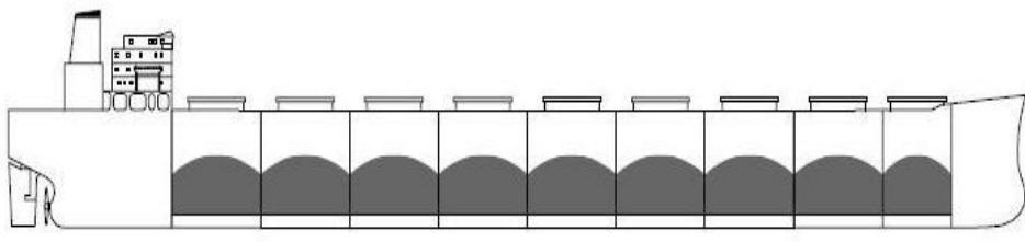
**Homogeneous Hold Loading Condition (Fully Loaded)**
