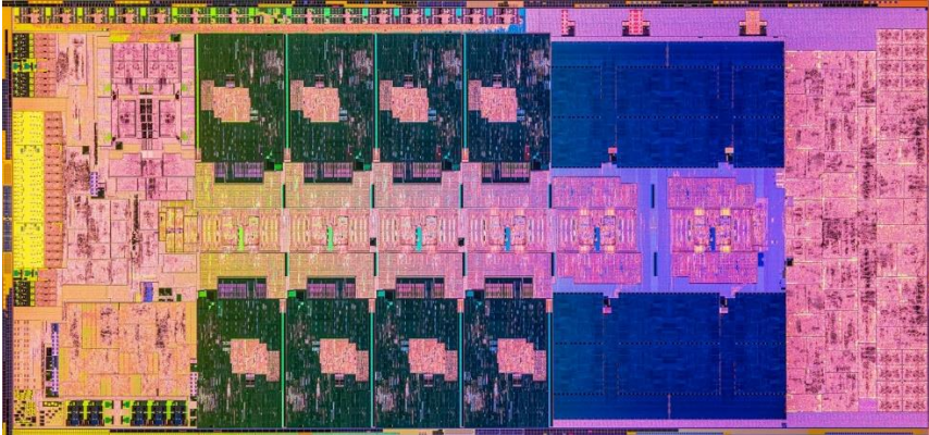
Slika 38.: Intel Raptor Lake Core (izvor: https://www.anandtech.com/show/17601/intel-core-i9-13900k-and-i5-13600k-review/2 )
