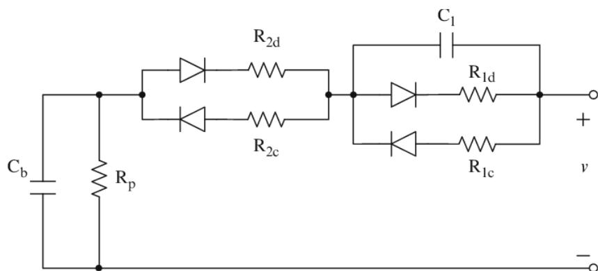
$C_b$  = battery capacitance,  $R_p$  = self-discharge resistance, or insulation resistance,
