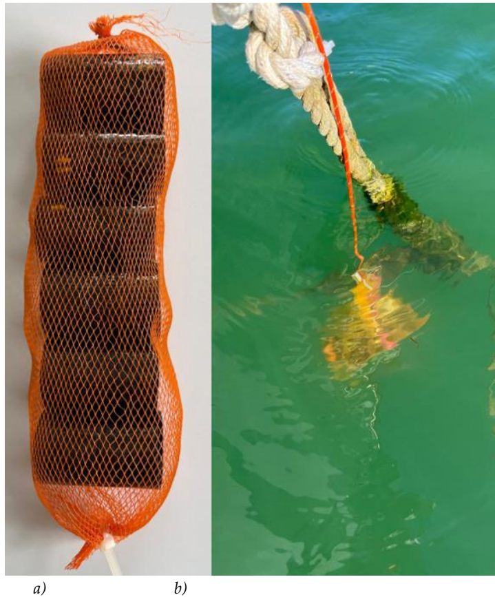
Figure 3 Specimens a) prepared, and b) submerged under seawater
