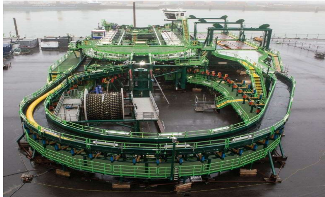
Slika 8. Cable Instalation Spread kabelopolagača Livingstone
