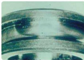
Stage 2: Surface distress and small cracks develop. Then microspalling occurs.
