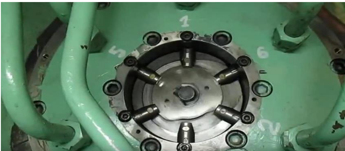
Figure 4 Starting air distributor
