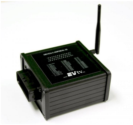
Slika 3.6. GEVCU (Generalized Electric Vehicle Control Unit)
