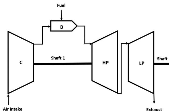
**Figure 2** The schematic view of gas turbine used in CODLAG propulsion system [26]
