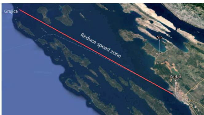
Figure 1 Reduce speed zone – pilotage of ships (Grujica-Zadar) [authors]
