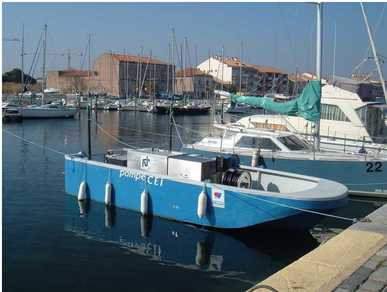
Image 2: Wastewater collection vessel from nautical vessels, yachts and boats Source: https://www.cei-marine.com/en/products/mobile-pumping-station.html , [Accessed on October 5 th 2021].
