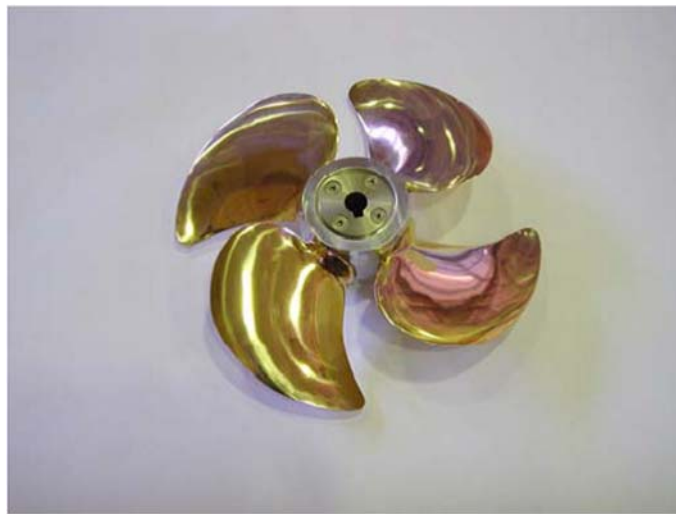
Slika 167: CPP propeler s broda RV Navigator XXI [4]
