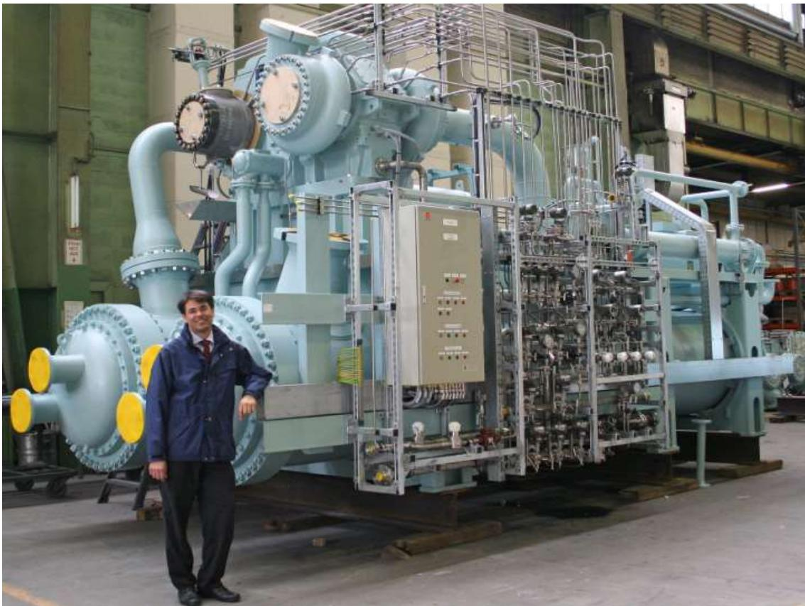
Slika 2: "Reliquefaction plant" [8]
