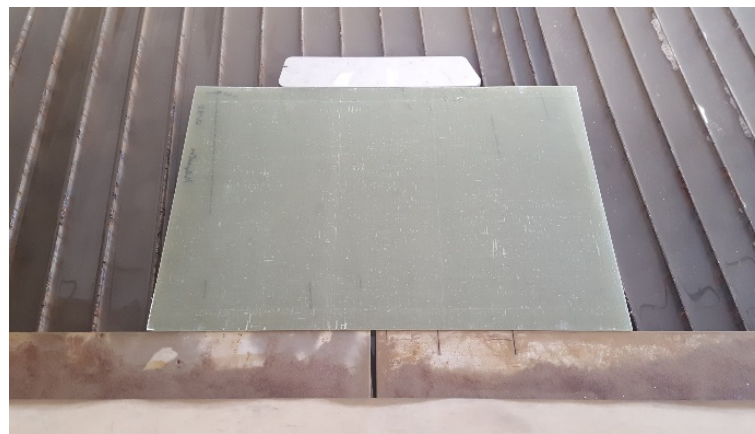
Figure 1. Composite plate prepared for waterjet cutting.
