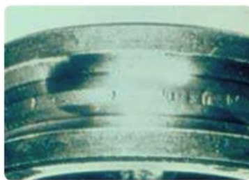
Stage 3: The debris is over-rolled; real surface spalling develops.
