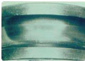
Stage 1: Fine roughening or waviness develops on the surface.
