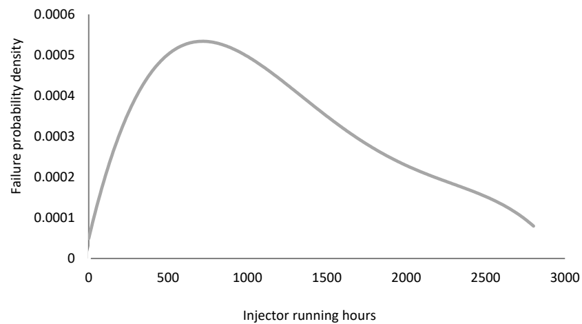
Figure 6. PDF for injector failures ( \beta = 1.46, \eta = 1446 ).
