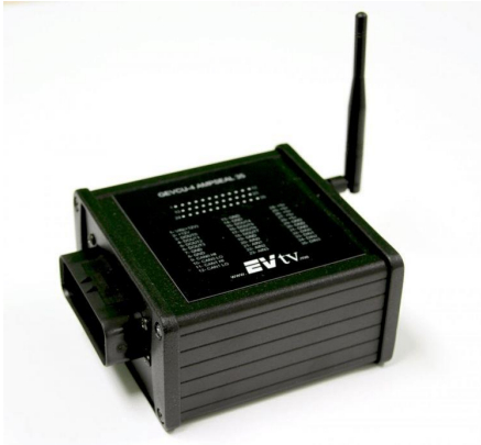
Slika 3.6. GEVCU (Generalized Electric Vehicle Control Unit)
