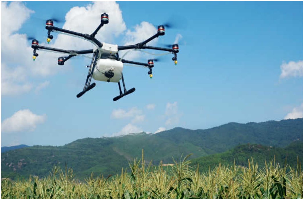
Picture 10: DJI MG-1 agricultural spraying drone
