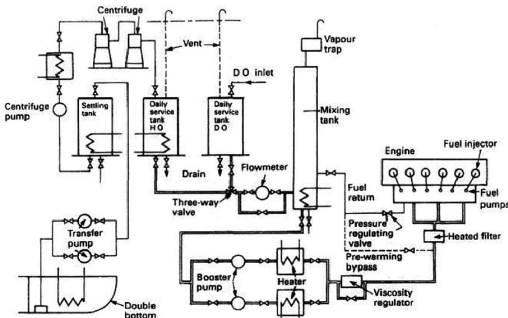
Fig. 2 Generic fuel system layout onboard a vessel
