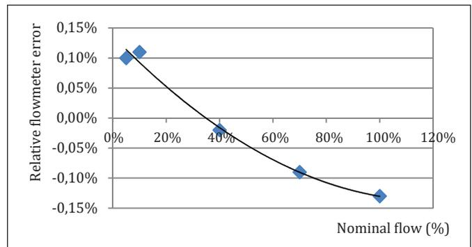
Fig. 9 Relative error of volumetric fuel flow vs. observed flow meter capacity – ship A
