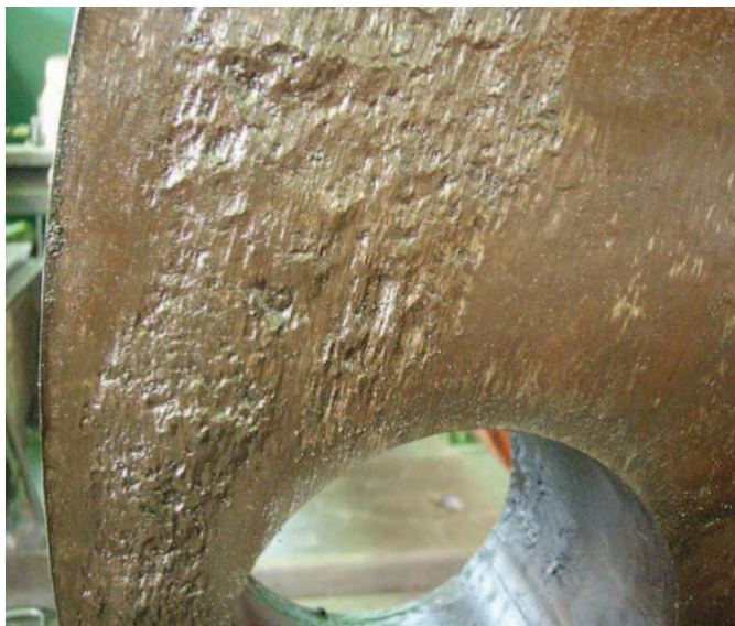
Figure 6 Fatigue Indicative Fretting on Surfaces [13]
