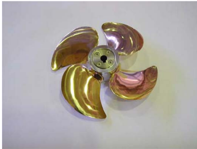
Slika 167: CPP propeler s broda RV Navigator XXI [4]
