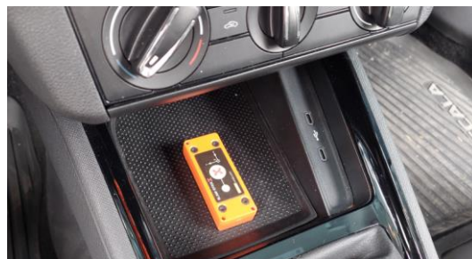
Figure 4. MEMS accelerometer position
