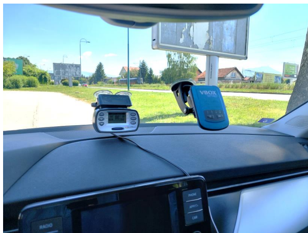
Figure 5. VBOX device setup
