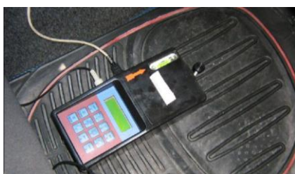
Figure 14. Decelerometer MAHA VZM 100
