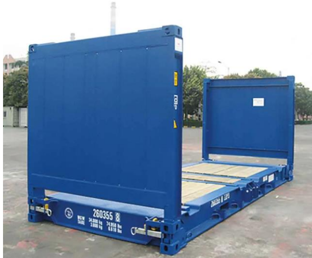
Slika 6. Flat rack container,
