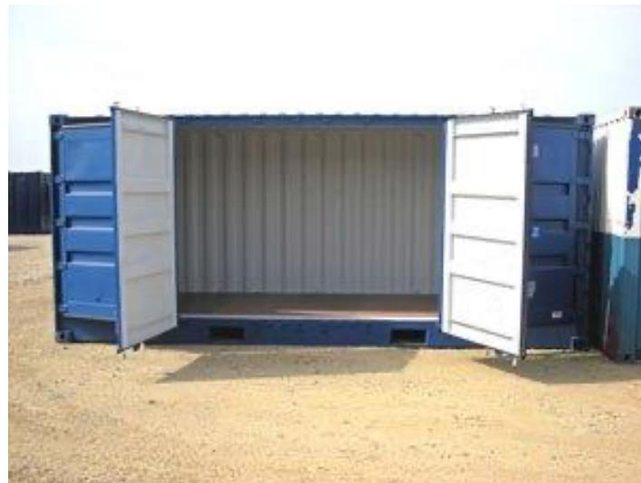
Slika 17. Kontejner otvoren sa strane. „Open side storage container“ (preuzeto sa: <https://www.marineinsight.com/know-more/16-types-of-container-units-and-designs-for-shipping-cargo/> )
