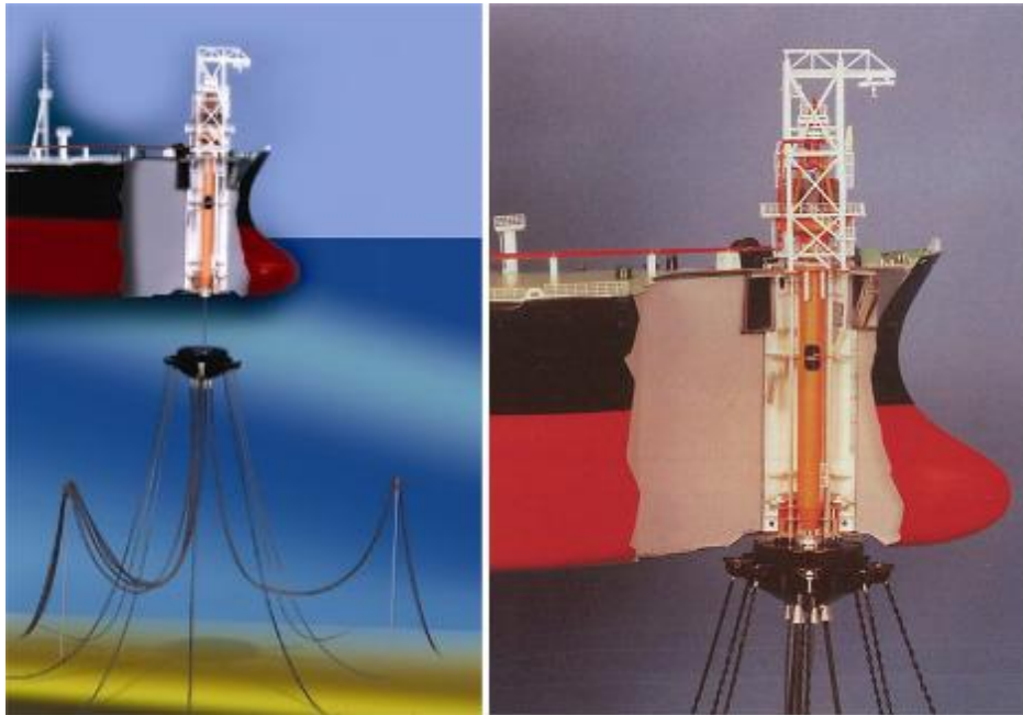
Slika 7: Internal turret mooring
