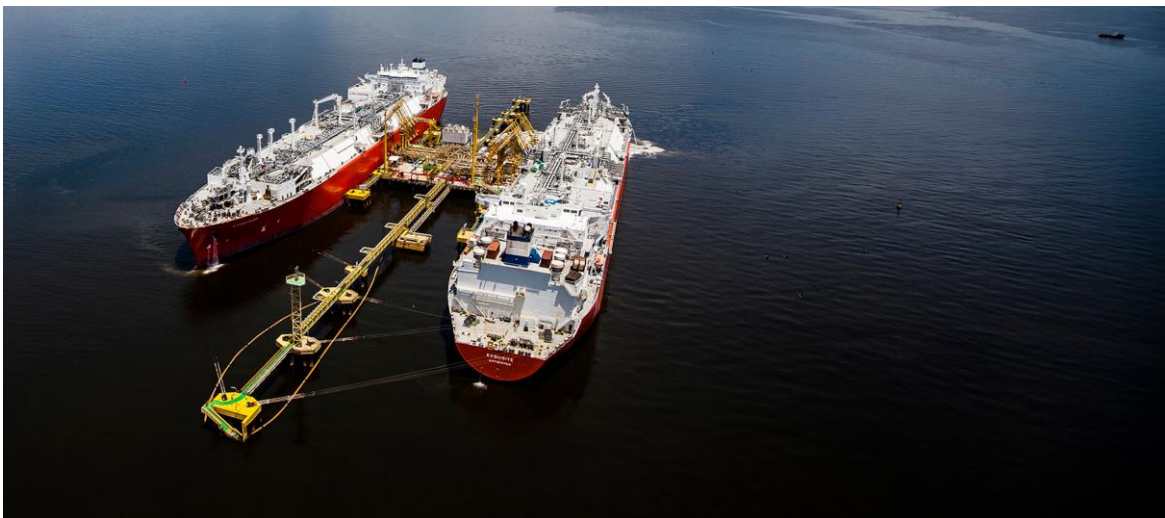
Slika 5: Cross jetty mooring
