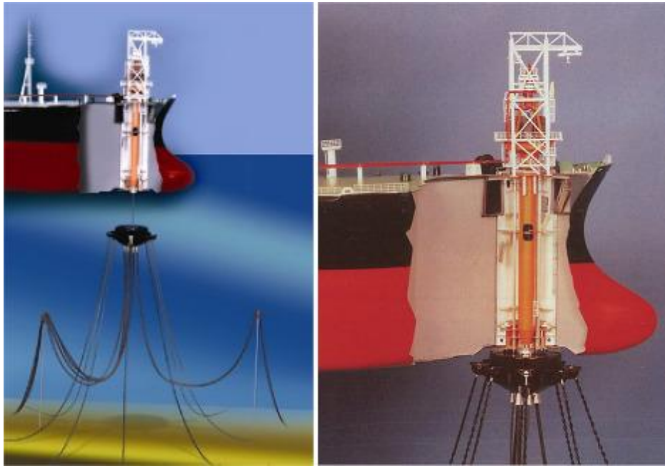
Slika 7: Internal turret mooring
