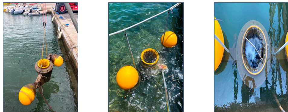
Figure 4. Seabin device installed in referring ports.
