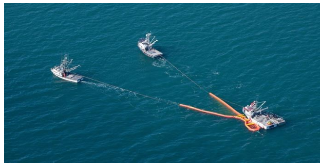
Figure 4. The example of a nearshore recovery system using a boom and a skimmer [19].
