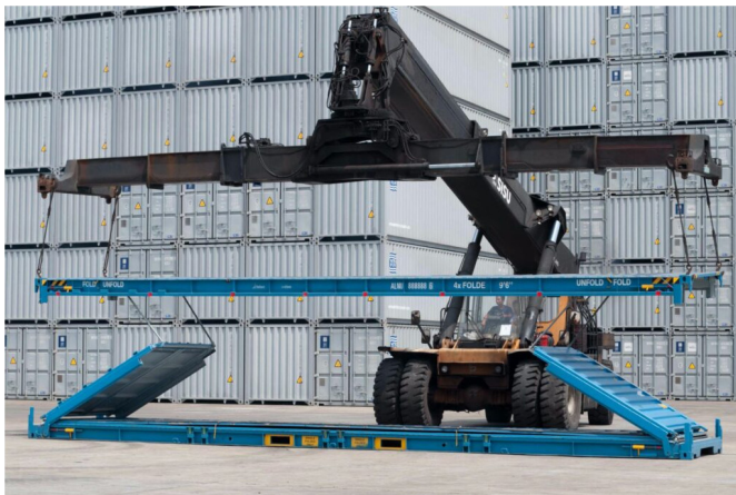
Figure 9 The folding process of the 4FOLD container [1]
