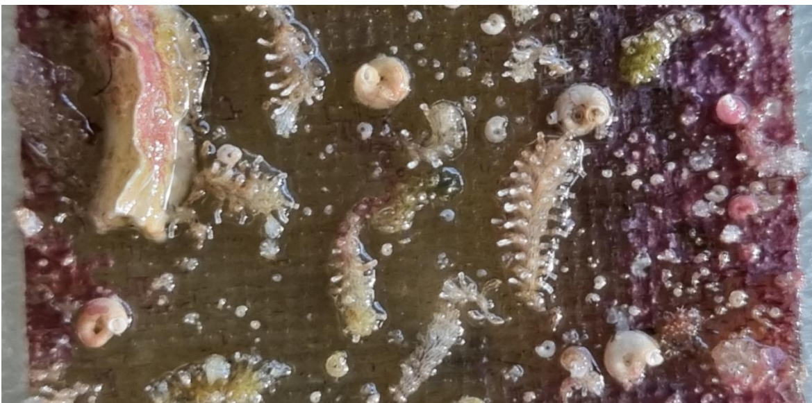
Fig. 3. Attached bio-growth after 24 months: a) entire coupon, b) detail optical zoom 3×; c) detail optical zoom 10×
