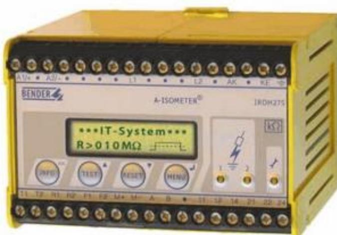
*Slika 28. IMD Insulation monitoring device*
