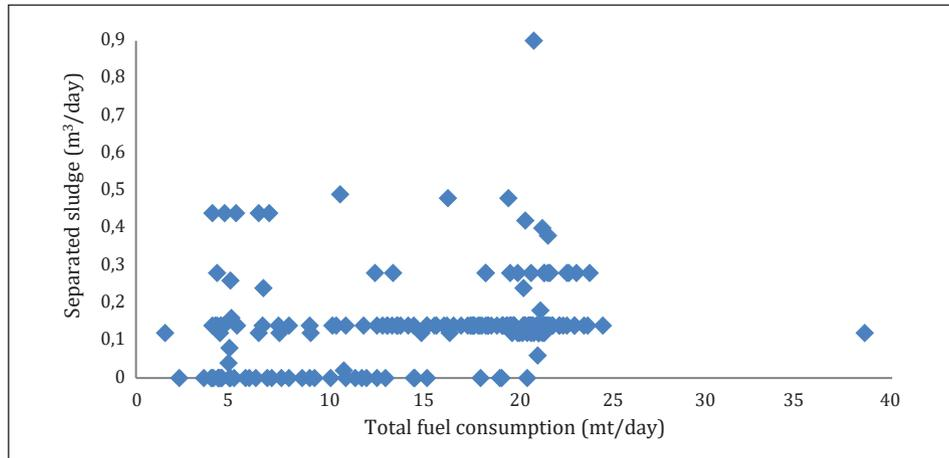
**Figure 6** Dependence of the separated sludge to the total fuel consumption for the period 02/2020 – 08/2020 – M/V Vessel
